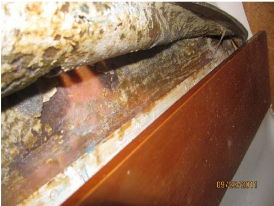
3 Beneteau First 210 Starboard Quarterberth, Exterior Damage Above Hull Pan Liner
